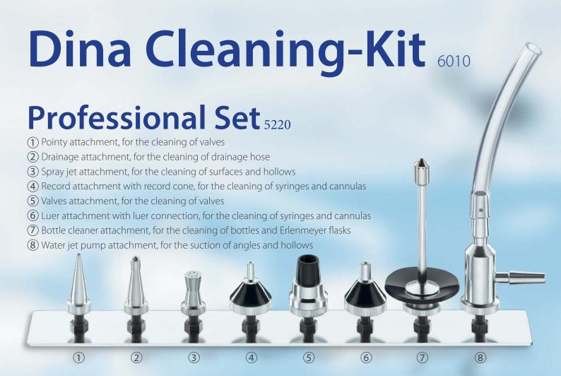
**HEGA** Rinsing Guns ensure with their good dosability a highly satisfactory result regardless of whether cleaning with water or drying with air. Using different attachments which only have to be plugged on, even the most remote corners can be reached. **HEGA** Rinsing Guns Dina and Nova have been designed and tested practice safe. Their tips lock the accurately fitting attachments and the standard cone keeps the attachments safe and clean in a table or wall mount.
